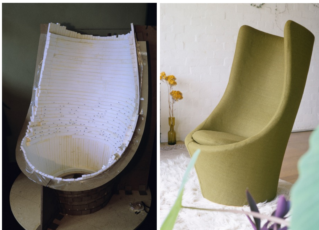
Left: Polystyrene prototype for the Expo '67 Talking Chair, 1966, photograph: Grant Featherston, Featherston Archive, National Gallery of Victoria Right: Expo '67 Talking Chair 1966, photograph: Grant & Mary Featherston, Featherston Archive, National Gallery of Victoria
